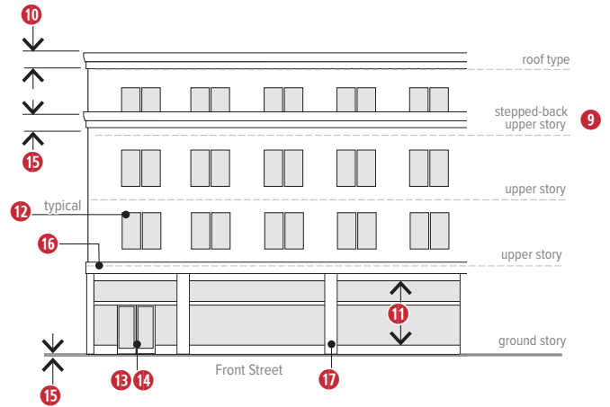
Figure (5) Storefront Building Street Facades
